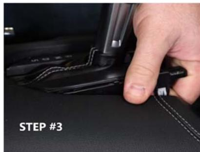
Step 3: Remove the base plate, that is held down by clips, by pulling up on the front and use a plastic pry bar to assist with the sides.
