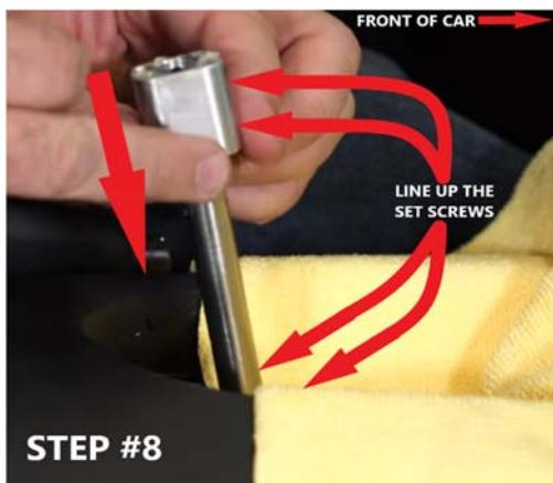
Step 8: Time to install the Shelby Shifter handle retainer. *Note: make sure to lay a rag or something down in the shifter location in the center console to prevent dropping the small screws.*
