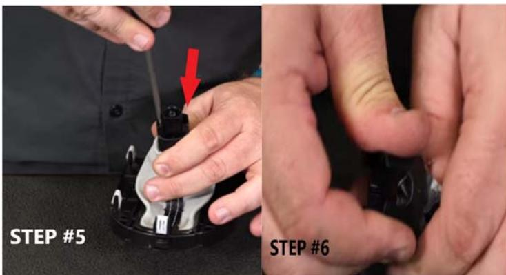
Step 5: Using a small flat blade screw driver, press on the two tabs on each side of the retainer, on the bottom of the shift handle, to release the shift handle from the shifter boot. The stock shifter handle is no longer needed. *Note: Use caution to not damage the shifter boot. It is reused.*
